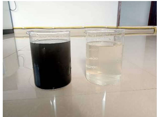
Left: Inlet from MPS | Right: Effluent Water
