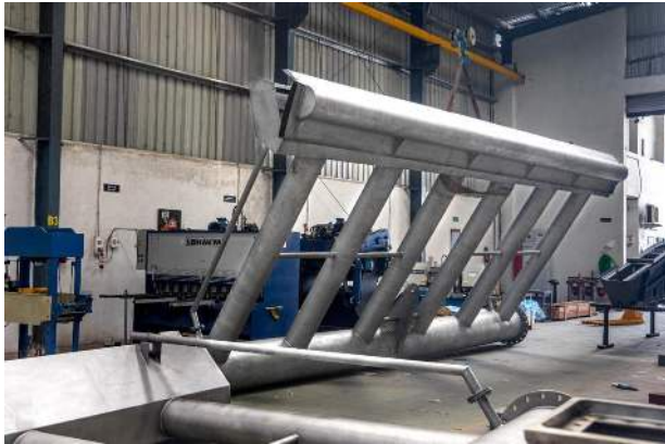
Photo: Batchflow decanter under manufacturing at Adroit's manufacturing facility Indore
